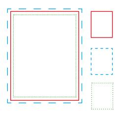
Finished page width 216mm (8.5") Finished page height 280mm (11") as per solid line on diagram
